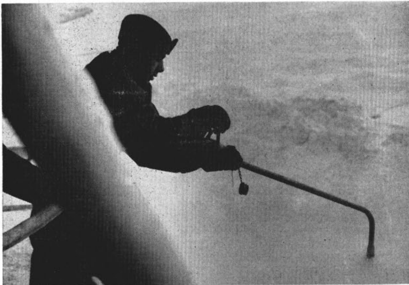
SPRAY GUN helps in removing ice. A mixture of steam and water on ice-coated areas is used to clear ship of 'frosting' in sub-zero weather.
