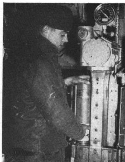
LOADING UP —Handler, above, puts 5-inch shell in a lift. Below: Shellman in mount takes it from the hoist.
