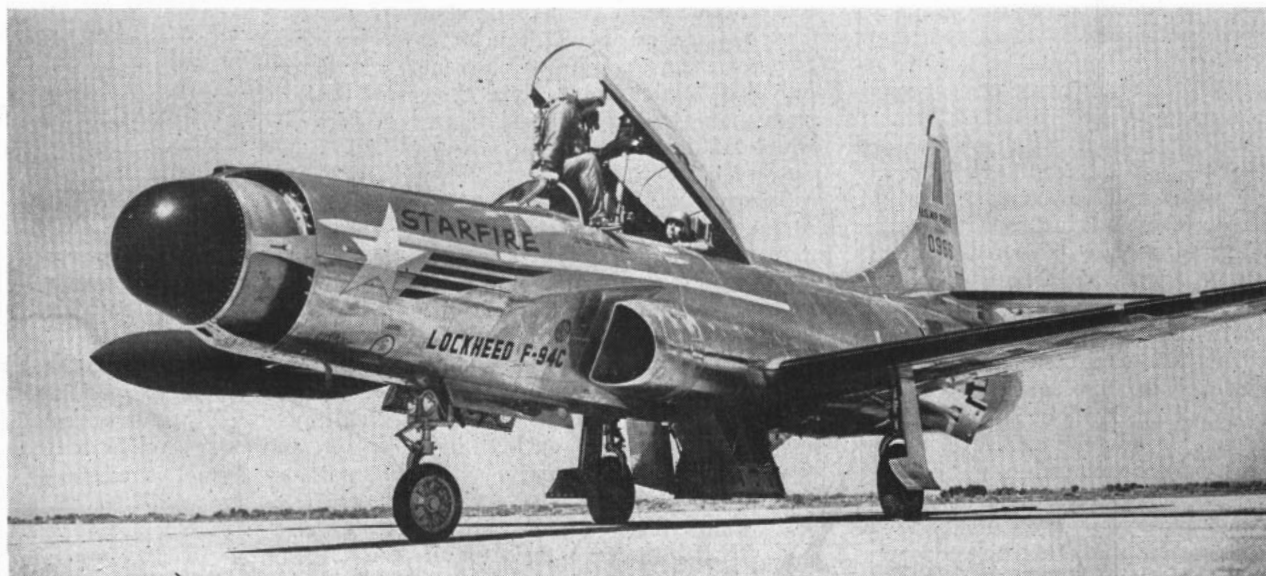
FIRST PLANE with all-rocket armament, Air Force's F-94C Starfire has 24 rockets, each able to blast a bomber from sky.
