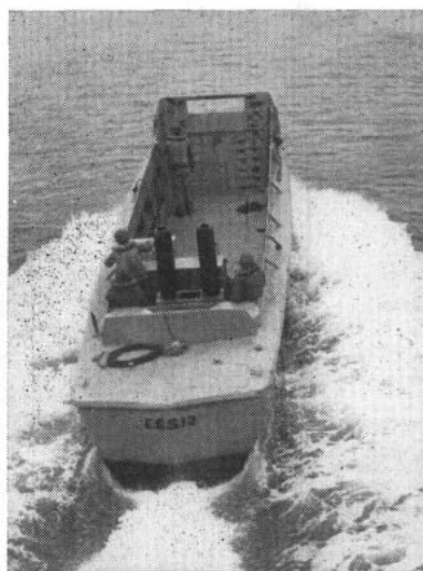
PEPPY new gas turbine engine has 160-horsepower potential, propels LCVP at 12-knot speed.
