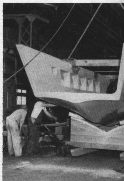
pears after it is removed from molds as a finished 'sandwich.' Right: The boat is put on a cradle for fitting-out.
