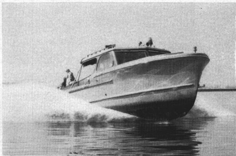
CABIN CRUISER is of all-plastic construction. Note (at right) how the ribs and keelson are molded right into the hull.
