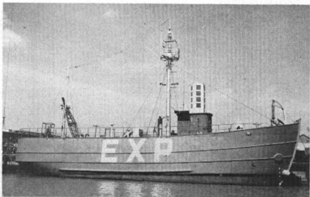
CREWLESS lightship being tested by Coast Guard may replace manned vessels guarding U. S. shipping lanes.
