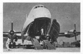
CLAM-SHELL loading doors permit wheeled vehicles to drive aboard AF's huge new C-124 Globemaster II. 3,500 horsepower at take-off. Weight of the plane itself is approximately 175,000 pounds. Its design calls for a cruising radius of 850 miles fully loaded, with a reserve of fuel to permit return to the starting point unloaded. A greater radius will be attainable when the plane is carrying lighter cargoes.
