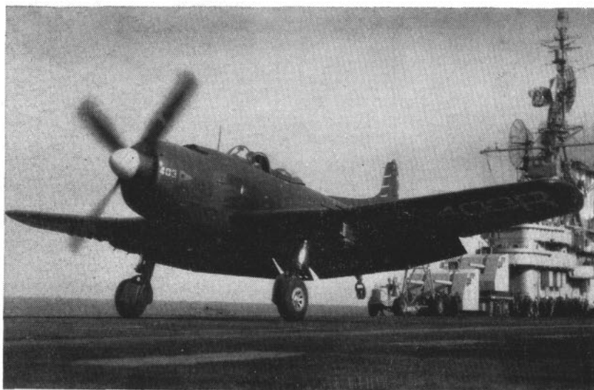
VERSATILE attack plane, faster and heavier armed than predecessors, AM-1 Mauler has passed carrier qualification tests on board USS Kearsarge (CV33).
