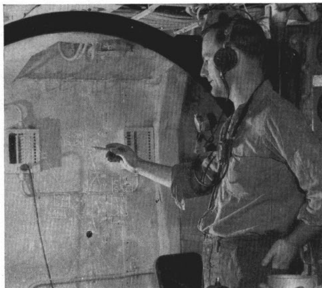
SIMULATED attack is plotted on dead reckoning tracer (left). Right: Data is recorded on the vertical plotting board.
