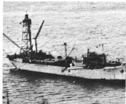
USS PATOKA —Unusual type ship was equipped to fuel, provision dirigibles.
