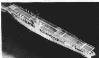
USS RANGER—First U.S. Navy vessel designed as a carrier, had six stacks.
