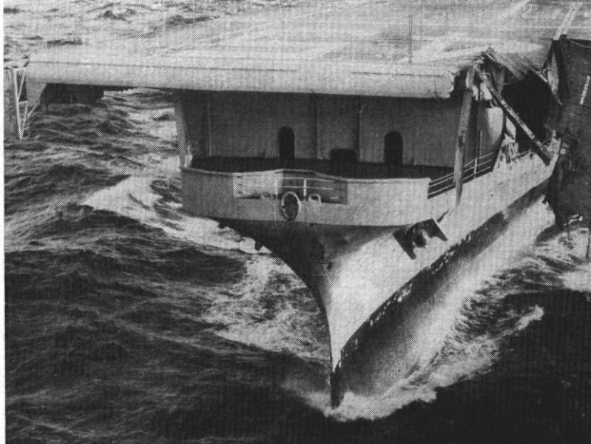
JAW BREAKER —Power of the storm-whipped sea is clearly shown by bow damage to USS Valley Forge (CVS 45).
