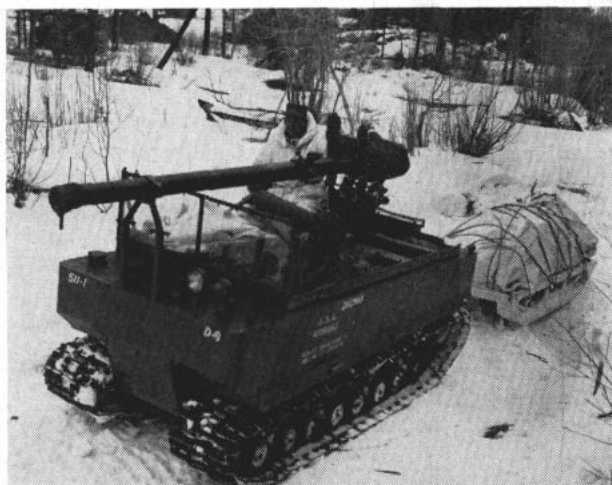
SLED DOG of the Army, the Arctic vehicle, Weasel, tows sled with ton of supplies. Gun is 105mm, recoilless rifle.
