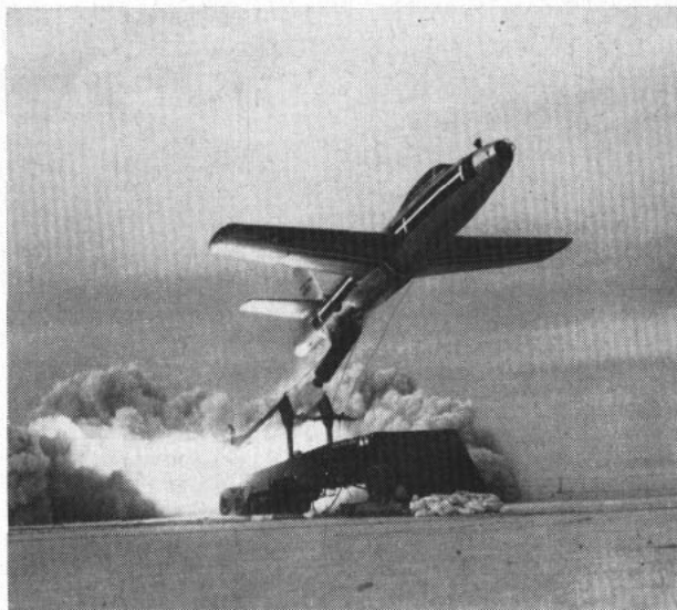
TRUCK-TOP TAKE OFF of conventional jet fighters is now possible with launching platform developed by Air Force.
