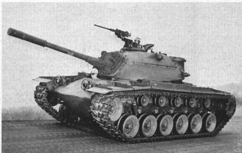
RAWIN, Army's radio wind system, permits continuous recording of atmospheric conditions as high as balloons can go. Right: Formidable fighting machine, 'Patton 48' tank has one-piece cast armor hull, better firepower.
