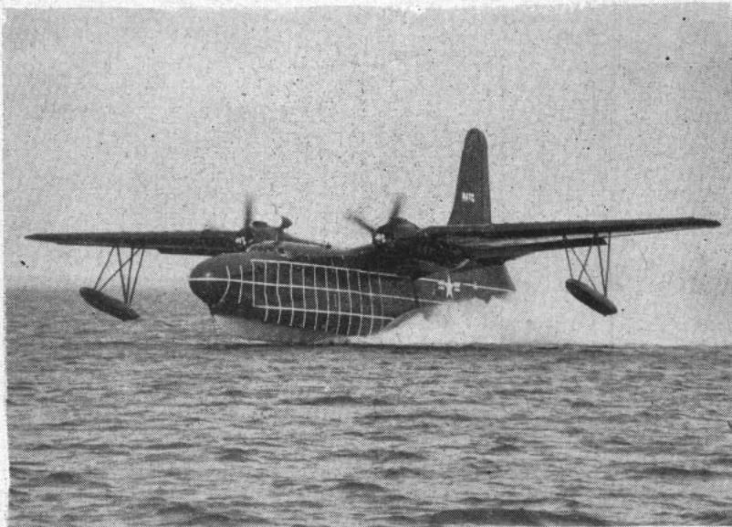
RADICAL hull, attached to the hull crown and wings of a World War II seaplane is now undergoing tests for possible future use with jet engines.
