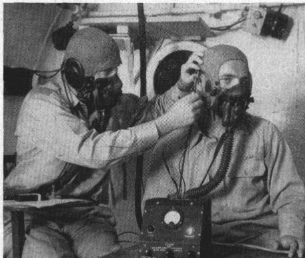
LIFE-SAVING OXIMETER, designed to warn flyers when oxygen supply is in danger, is being tested by USAF.
