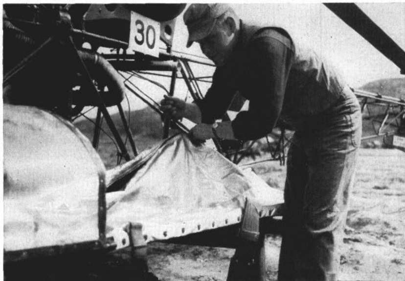
INVENTIVE MARINE, S/Sgt Arthur L. Kent, zips up a new litter cover he adapted from 'copter rotor blade cover to aid in casualty evacuation.
