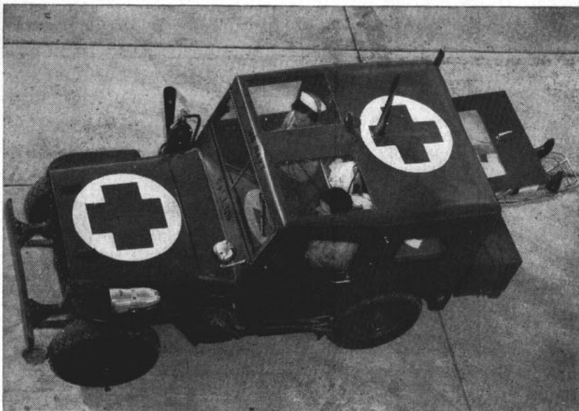
COMBINATION ambulance carrier-crash truck-radio car speeds up rescue work. Two plexiglas roof windows enable driver to spot rescue planes easily.
