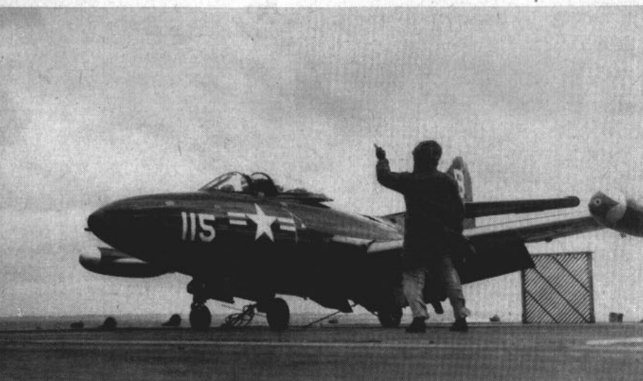
REVVING UP his F9F Panther jet, a pilot awaits the 'Fire!' signal from the catapult officer. Note the blast screen used to deflect the hot exhaust fumes.
