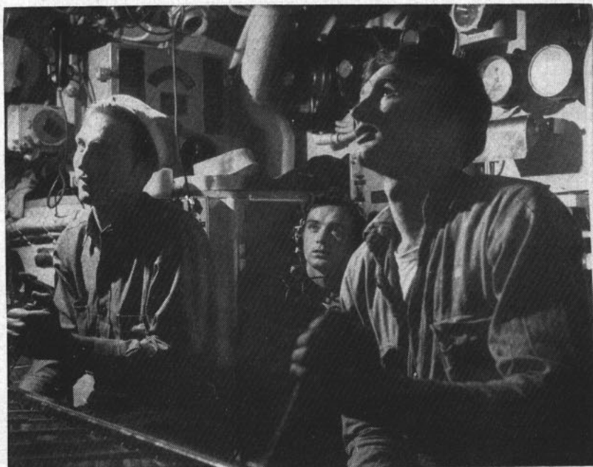
CONTROLLERMEN in the maneuvering room have the important job of regulating the speed of the ship on orders over the annunciators from the conn.
