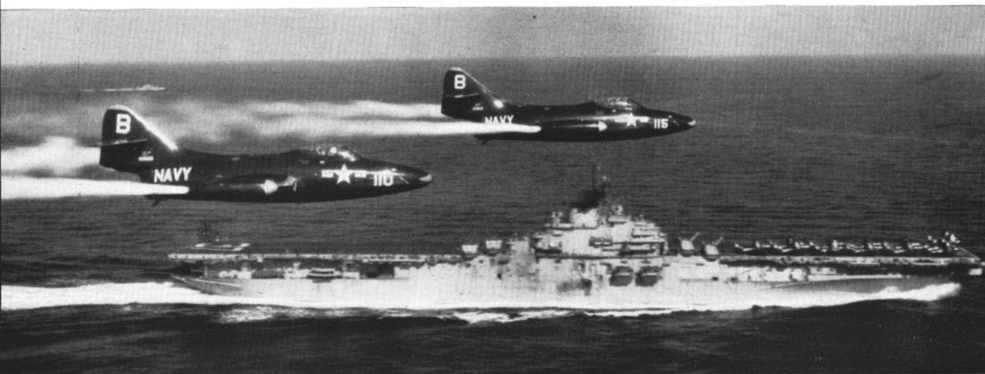
PANTHER JETS jettison unused gas prior to landing aboard Princeton . Gas left in plane is a potential fire hazard.
