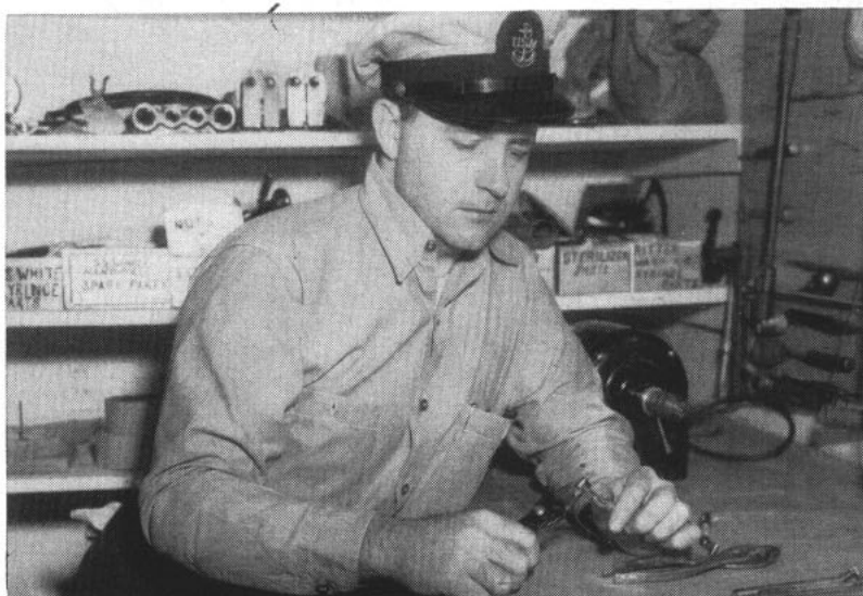
AGILE FINGERS of John Condrey, DTC, disassemble a drill which has been sent to him for repair. After overhaul, drill will be returned to its ship.
