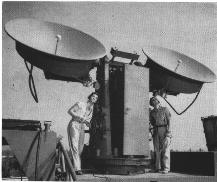
PROBING FINGER of radar tracks missile as it arches into space. Making use of the Doppler Effect, this unit can tell speed of missile at any instant.
