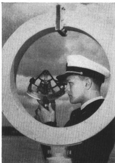
SEXTANT-TYPE stadimeter is operated by a cadet-midshipman during one of his periodic training cruises.
