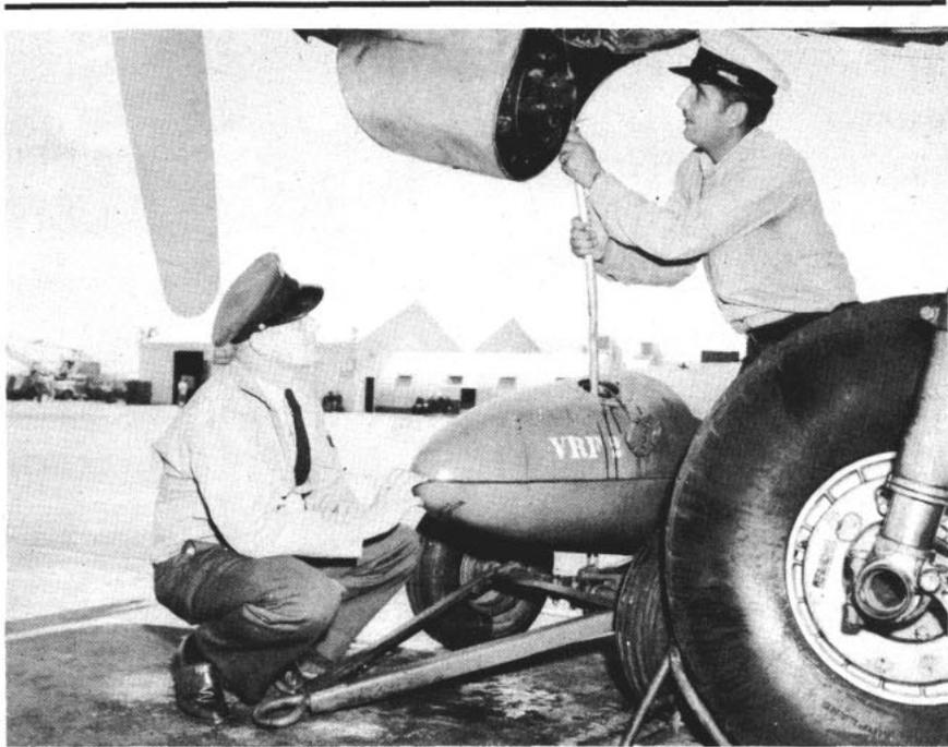
OIL BOWSER is name of contraption being used by its designers at NAS, San Diego, to drain oil safely from aircraft engine. Device came from the junk pile.
