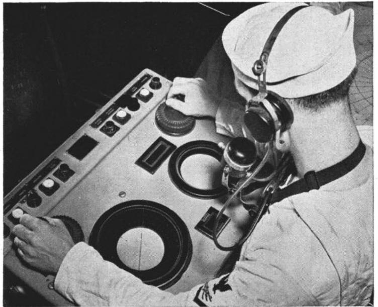
**TRANSMITTER** on board a cruiser is operated by radarman (left). Scope of ship's radar is eyed by operator at right.
