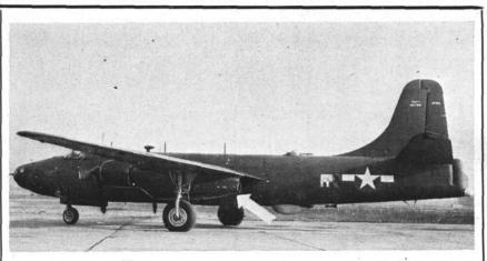
XP4M-1 is powered by two huge conventional engines and two jet engines in two nacelles. Arrow points to jet engine mounted behind conventional engine.
