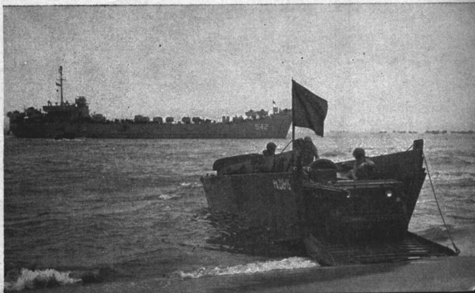
SMALL SUPPLIES are brought in immediately after assault waves. LCVPs like this one (below) bring materiel to set up command posts, medical units.
