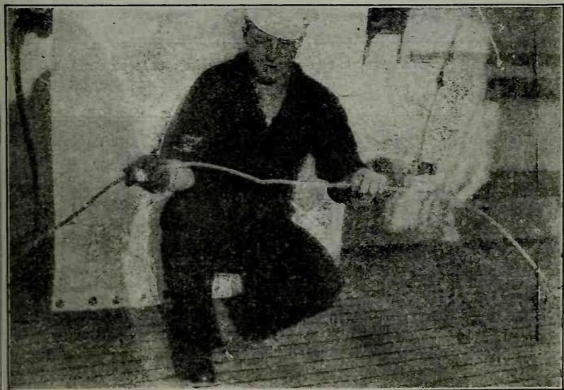
FIG. 47-7—The correct way to take a kink out of wire rope, fourth step.
