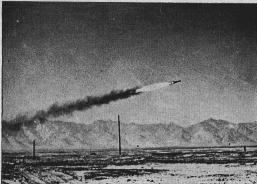
'FLYING STOVEPIPE', Navy's working model of ram jet propulsion, streaks from its platform in test hop which may usher in era of 1,500 mph flight.
