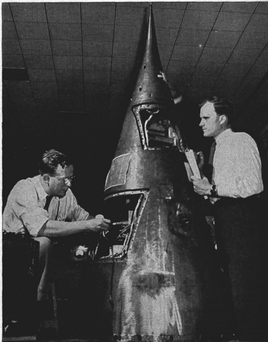
Official U. S. Navy photograph MINIATURE LABORATORY, constructed in the warhead of a V-2 rocket, gets a final checkup before the rocket is fired into the air at Las Cruces, N. M.
