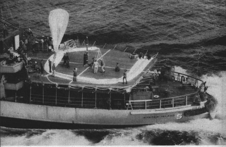
GOING UP! Helium is pumped into 'Skyhook' balloon. At center of deck is 'Deacon' rocket, soon to be carried aloft.
