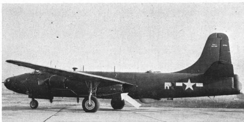
XP4M-1 is powered by two huge conventional engines and two jet engines in two nacelles. Arrow points to jet engine mounted behind conventional engine.
