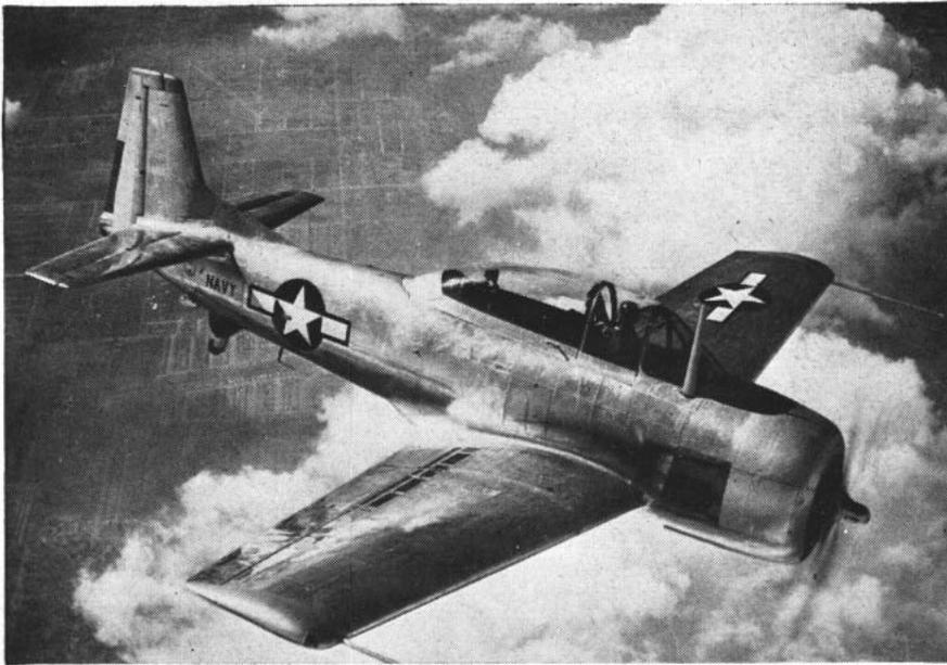
XSN2J-1, experimental intermediate trainer developed by North American, has a top speed of 270 miles an hour. The Navy has ordered the plane for evaluation.
