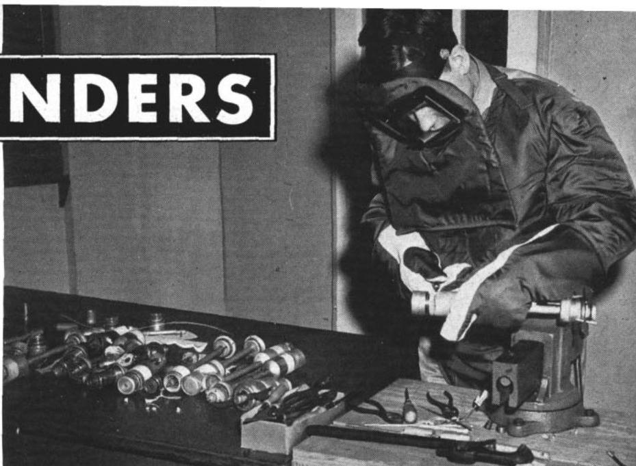
PROTECTION suit of 78 layers of nylon and mask containing viewing part of shatterproof glass are worn by man stripping fuze from the arming pin.
