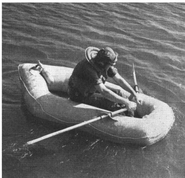
(4) A pair of collapsible oars are stowed aboard the raft. The pilot inserts oars in oar-locks and he is away.
